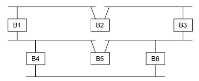
Here's one. Note that the Spanning Tree we're looking for must include ALL of the networks – the bridges don't have to be included
