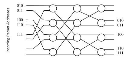
b) Show which output link each of the incoming packets is routed to in this Batcher switch:
