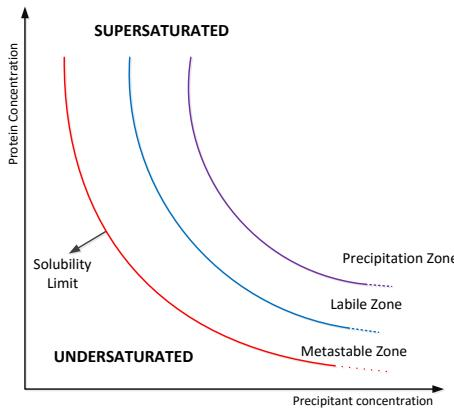
Fig. 1. Phase Diagram.
