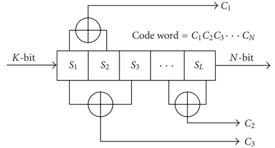
FIGURE 2: Encoder block (shift register) using convolutional codes.
