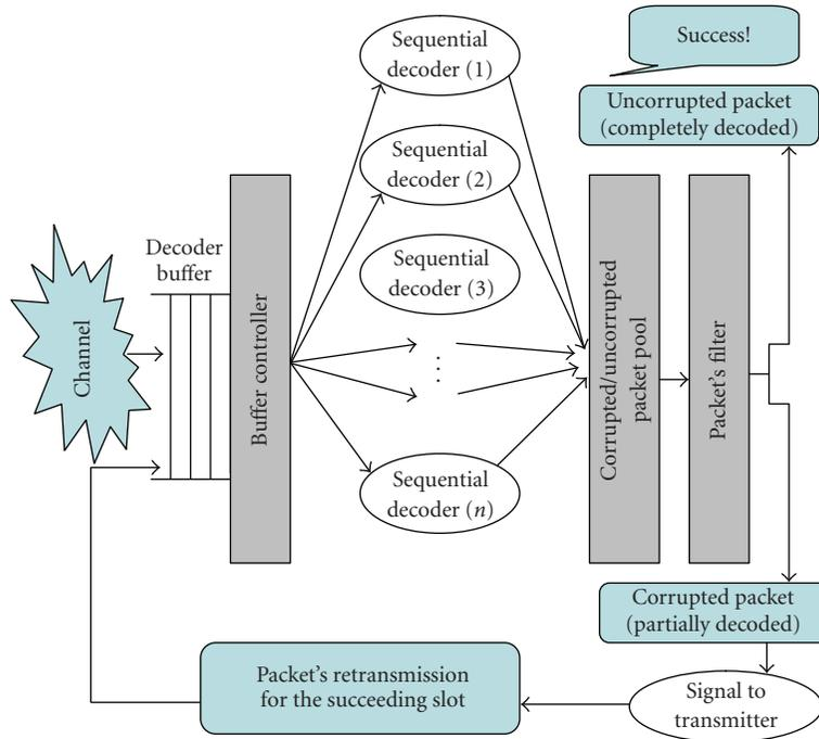
FIGURE 10: Router system with parallel sequential environment and single address space structure.
