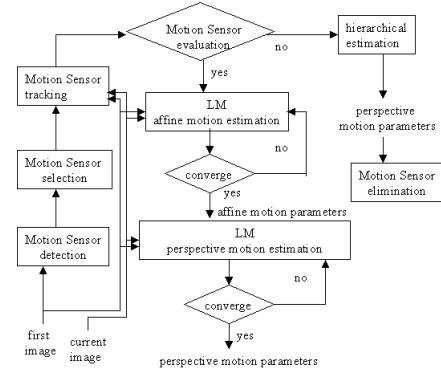
**Fig. 4.** Global Motion Estimation Algorithm.
