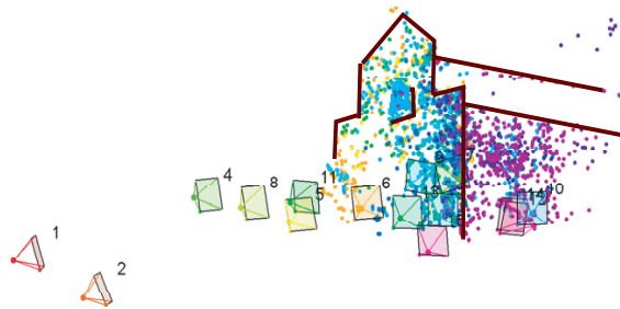
Fig. 10. Another view of the reconstructed 3D scene and camera configuration for the real experiment. Reference lines are superimposed on the image for better perception. The viewpoint is roughly similar to image 9 in Figure 8.
